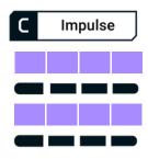
"Impulse" is for short and intense sessions. Since all chambers are pulsed at the same time, "Impulse" maximizes the number of possible compression passes in a given time.
